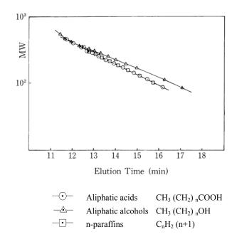
Fig. 2 Calibration curves for n-paraffin, aliphatic acid, and alcohol
