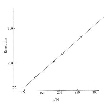
Fig. 7 Effect of number of theoretical plates on DEP-DMP resolution
