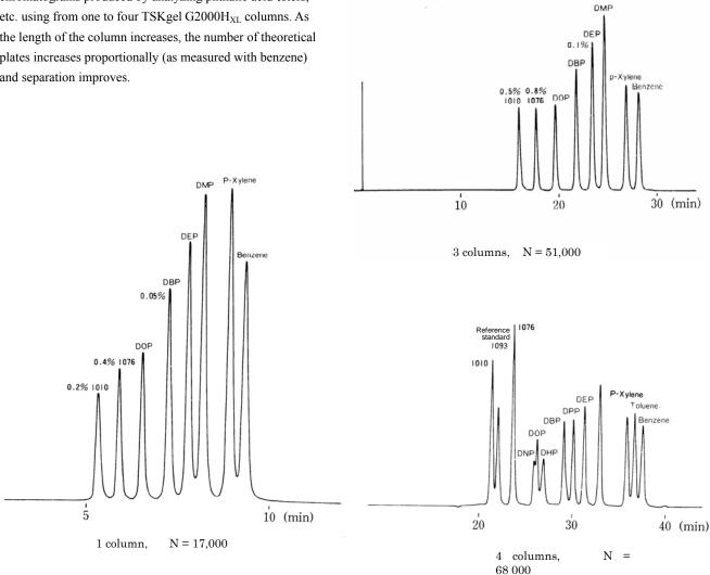
Fig. 6 Separation of phthalic acid esters by TSKgel G2000H<sub>XL</sub>
