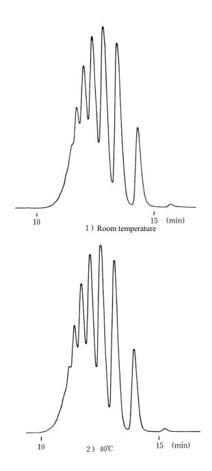
Fig. 11 Effects of column temperature on separation
