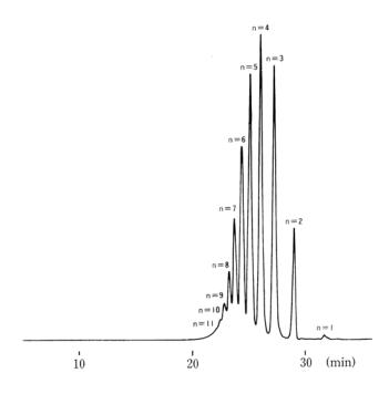
Fig. 10 Separation of A-500 using four G2000H<sub>XL</sub> columns
